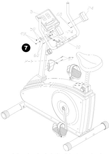
7. Attach the pulse wires in the handlebar (10) to the wires from the console (5). Connect the handlebar (10) to the console tube with the locknuts (49), flat washers (50) and screws (55) provided. Make sure not to "pinch" any of the pulse wires when connecting the handlebar to the console tube. Attach the elbow pads (24) to the handlebar (10) with screws (60). Attach bottle rack (2-1) to console tube (2).
